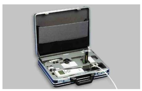
The DSS70A provides a compact solution for field checking dew point where direct measurement is difficult. Typical applications for the sampling system are metal treatment and plastics drying processes. (The DSS70 includes the sampling system and case, but not the MI70.)
