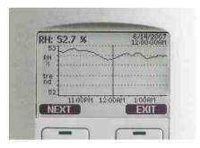
The display shows measurement trends and over four years of real-time measurement history.
