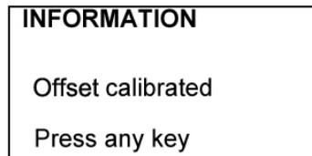
If in the installation is not possible to stop the flow rate, an offset adjustment can be done if the flow rate is stable.
