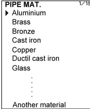
In the event that the pipe material is not on the list, you must select “Another material”, in the last position in the list. In this case, the sound propagation velocity of the material must be entered.
