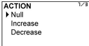
If "Null" is selected, the totalizer remains unchanged. If "Increase" is selected, the totalizer will add the amount of fluid passing through the flowmeter, and if you select "Decrease", the totalizer will subtract that amount.
