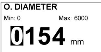
The outer diameter value must always be entered in millimetres.
