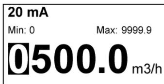
Programming a flow rate value for 20 mA higher than the one for 4 mA, the loop current changes from 4 to 20 mA as the flow increases.
