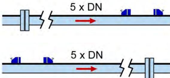
Some plant elements such as pumps, valves, etc., can create turbulences that distort the flow profile resulting in incorrect measurements. In this case, the distances of straight pipe without disturbing elements before and after the transducers can be higher, as shown in the following pages:
