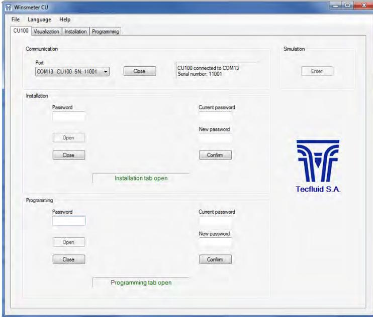
Once the password is written, press "Enter" or the corresponding "Open", and the installation or programming tab will open as appropriate. At the bottom of each section displays "Installation tab open" or "Programming tab open."
