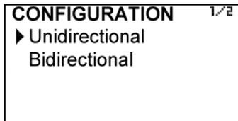
If "Unidirectional" is chosen, the analog output will have a value proportional to the flow rate when positive, and it will provide always 4 mA when negative.
