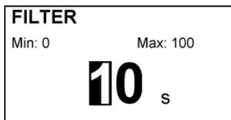
Only the flow rate indication of the display and the analog output are affected by the filter. The relay output and the totalizer act according to the instant flow rate. Selecting a filter with a longer or shorter integration time will provide more or less stable readings and will also affect the response time to small variations of flow rate.
