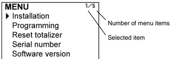
The "Installation" option allows the installation of the transducers, as explained in Chapter 5 of this manual.
