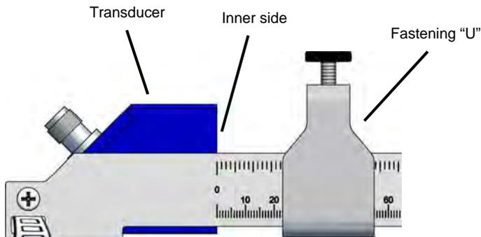
After placing the transducer, move the fastening "U" to it until the knurled screw matches the transducer top notch.
