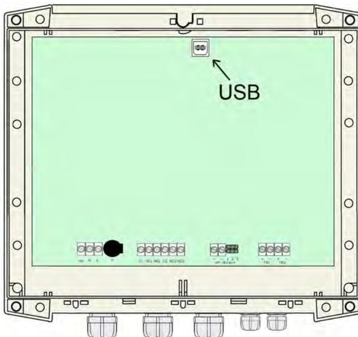
To open the lid, remove the four screws. The USB connector is located on the opposite side of the cable entry glands.
