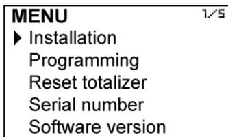
In order to access to the transducers installation menu, a password must be entered. When accessing the first time, the default password is 0123. For more details about the password, see paragraph 4.1, page 11.
