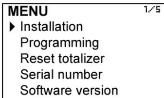
With the keys (2) and (8), select Programming, and then validate with the key (OK). To access the programming of the converter, you must enter the password. At first access, the default password is 0123. For more details about the password, see paragraph 4.1, page 11.
