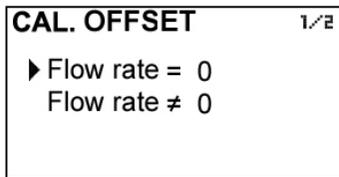
If the first option to make the correction is chosen, the flow rate must be zero, that is, the liquid inside the pipe where the transducers are installed should be completely stopped.
