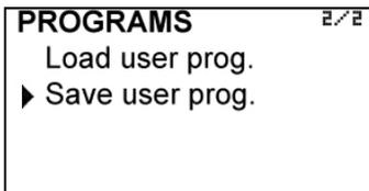
If at any time you want all the transducer installation data to be stored in memory as backup, it can be done by selecting "Save user prog. ".
