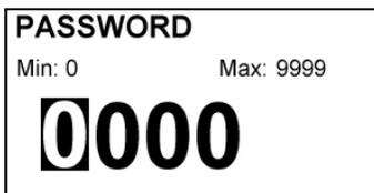
Once the password is entered, the first screen allows to choose between the different programming options.
