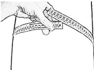
$$\text{Pipe diameter (mm)} = \frac{\text{Pipe perimeter (mm)}}{3,14}$$
