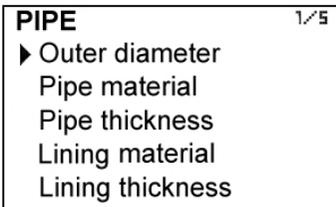
First, the outer diameter of the pipe must be entered.
