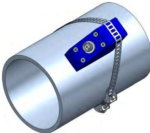
Place the transducer cables by screwing the connectors, and taking into account that the cable TR1 must be connected to transducer TR1 and the cable TR2 to the transducer TR2.
