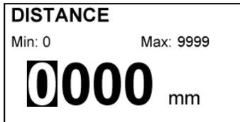
If the transducers have been placed by means of the fine adjustment of signal strength (paragraph 5.13), it is necessary to enter the practical distance at which the transducers have been placed. This distance will be shown on the installation screen (see paragraph 5.11) as Dp.
