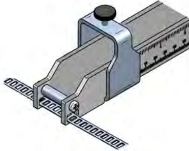
Place the strap encircling the pipe, positioning the free end over the hooks and below the screw. Snap the hooks on the tightest position possible. Tighten the connection with a screwdriver until the guide is fixed rigidly, with no possible movement due to vibrations.
