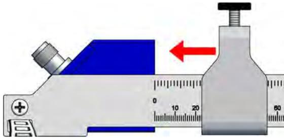
Once in this position, tighten the screw until the transducer is pressed against the pipe.
