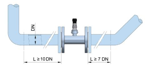
These distances can be reduced by installing a flow straightener upstream of the turbine at a distance equivalent to 5 DN.
