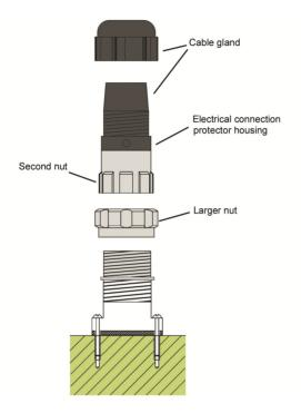
Loosening the larger nut in the middle of the connector allows us to withdraw the half where the cable will be later soldered.
